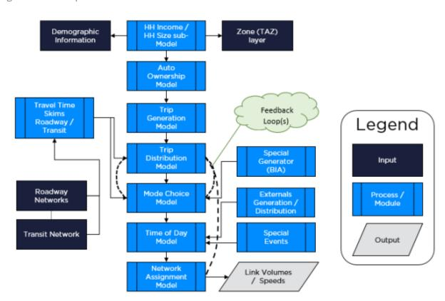
Figure 3: Four-Step Process in TDM
